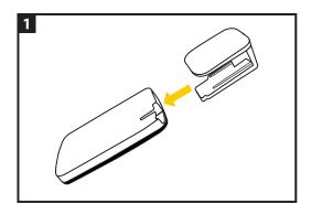
1. Attach the bracket to the transponder by sliding it into the slot of the transponder until it clicks in place.
